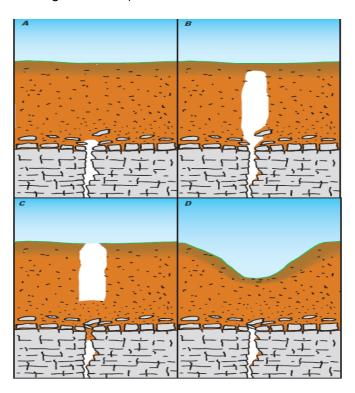
**Figure 3-15:** Formation of collapse—Soil bridges gap where sediment has been washing into a solution enlarged fracture, A. Over time, the void migrates upward through the soil, B. After the bridge thins, a sudden collapse, C, often plugs the drain and erosion will, after many years, transform the collapse into a more bowl-shaped sinkhole, D.
