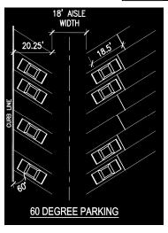
*Note*: Two-way drive aisles shall always require a minimum width of 24 feet.
